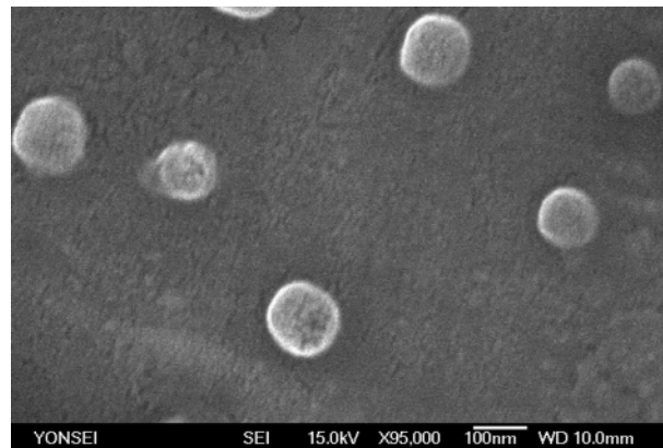
Figure 6. SEM image of the capsules formed by 7a ( 5 \times 10^{-3} g/mL) in H 2 O in the presence of CHCl 3 ( 1 \times 10^{-2} mL/mL).
